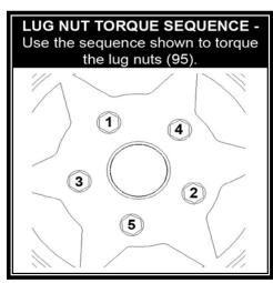
**WARNING:** Retighten lug nuts at 500 miles after any wheel change, or anytime the lug nuts are loosened. Failure to do so could cause wheels to come off while vehicle is in motion.
