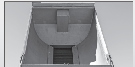
Unique, roll-formed sides and cross memberless floor design
