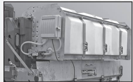
LS4T (tailgate mount 105 gal. poly reservoir)
