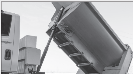
Mailhot® multi-stage, double-acting, nitrided cylinder, trunnion-mounted hoist
