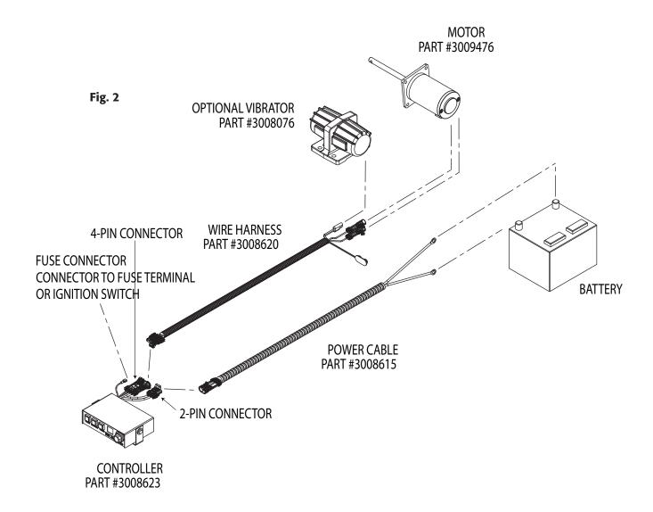
Observe spinner direction of rotation. The correct direction is counter clock wise when looking inside hopper from the top. If direction is clock wise reverse wires between Motor and Wire Harness.
